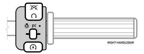
**NEUTRAL ON** + (7) ENGINE ON + **CLUTCH ON**
